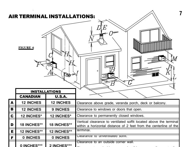
Clearance to an inside non-combustible corner wall or protruding
