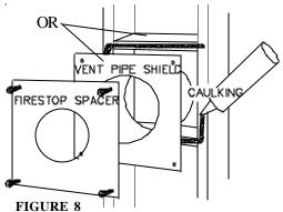
1. Mark and cut the vent pipe shield to the determined depth of the combustible wall. Apply a bead of caulking (not supplied) to the framework or to the shield plate (in the case of a finished wall) and secure the shield through the opening to the interior wall. The final location of the vent pipe shield should maintain the re-
