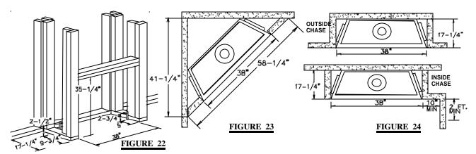
It is best to frame your fireplace after it is positioned and the vent system is installed. Use 2x4's and frame to local building codes. **FIGURE 22-24.** To install the fireplace face flush with the finished wall, position the framework to accomodate the thickness of the finished wall. Pull out the four nailing tabs, attached on either side of the fireplace and secure to the 2x4 framing to facilitate drywall installation.
