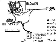
INSTALLATION TO BE DONE BY A QUALIFIED INSTALLER and must be electrically connected and grounded in accordance with local codes. In the absence of local codes, use the current CSA C22.1 CANADIAN ELECTRICAL CODE in Canada or the ANSI/NFPA 70-1996 NATIONAL ELECTRICAL CODE in the United States.
