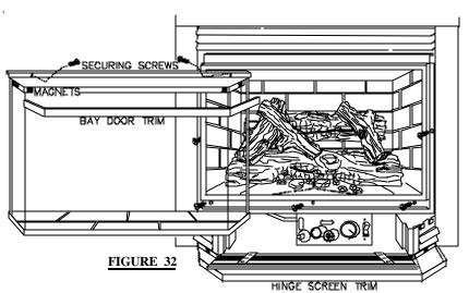
LOUVRES: Install the louvres and louvre assemblies as illustrated in **FIGURE 31**. The bay door trim is attached with magnets.
